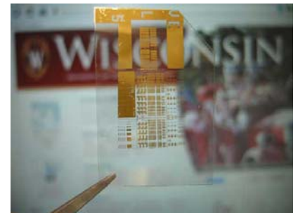
A thin-film transistor (TFT) made with silicon nanomembranes. TFTs are the basis for flexible electronics.
